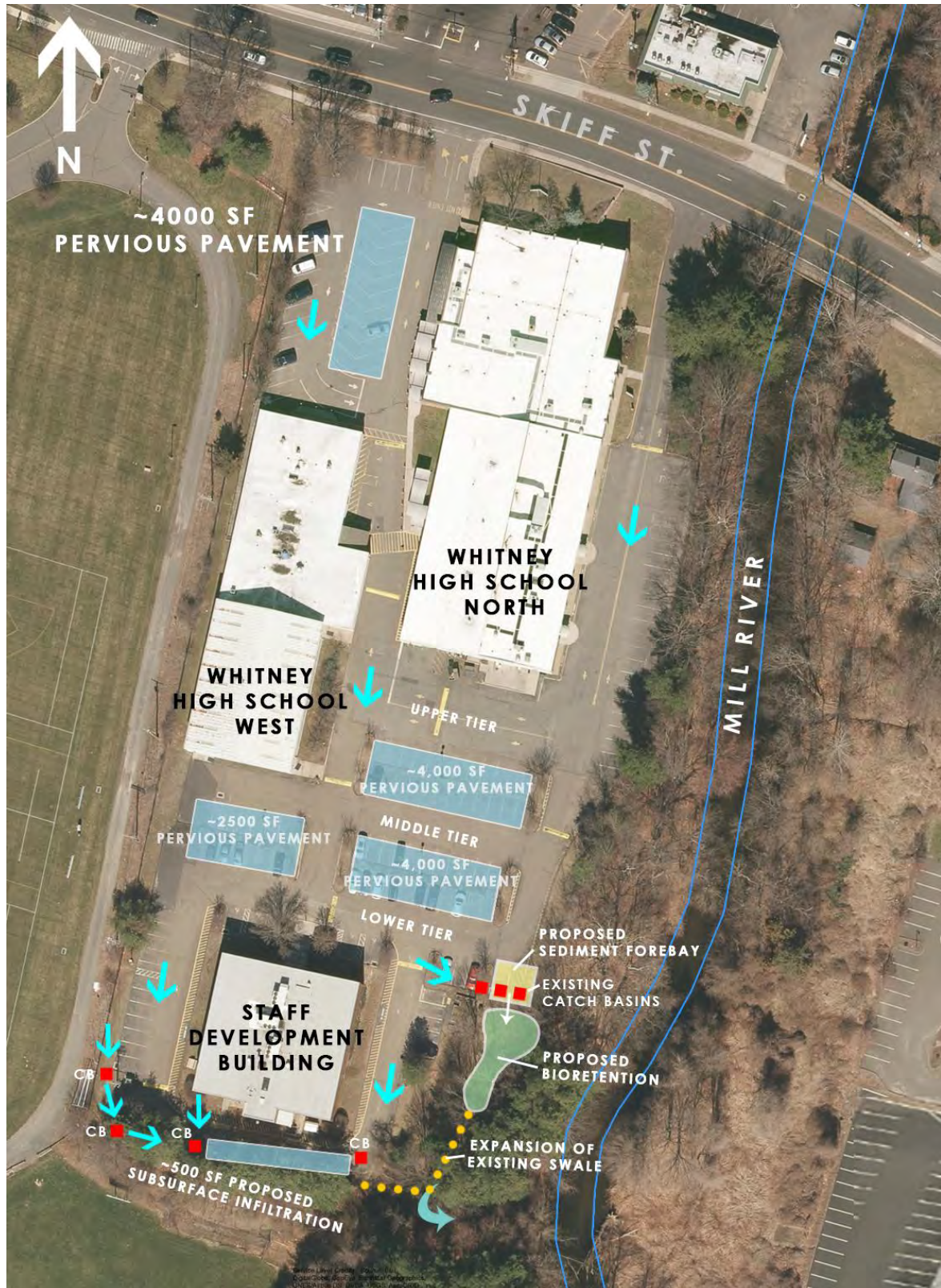
Figure 19. Proposed green infrastructure retrofits for Whitney High School North/West. "CB" indicates existing catch basin. Blue arrows indicate existing surface flow patterns.
