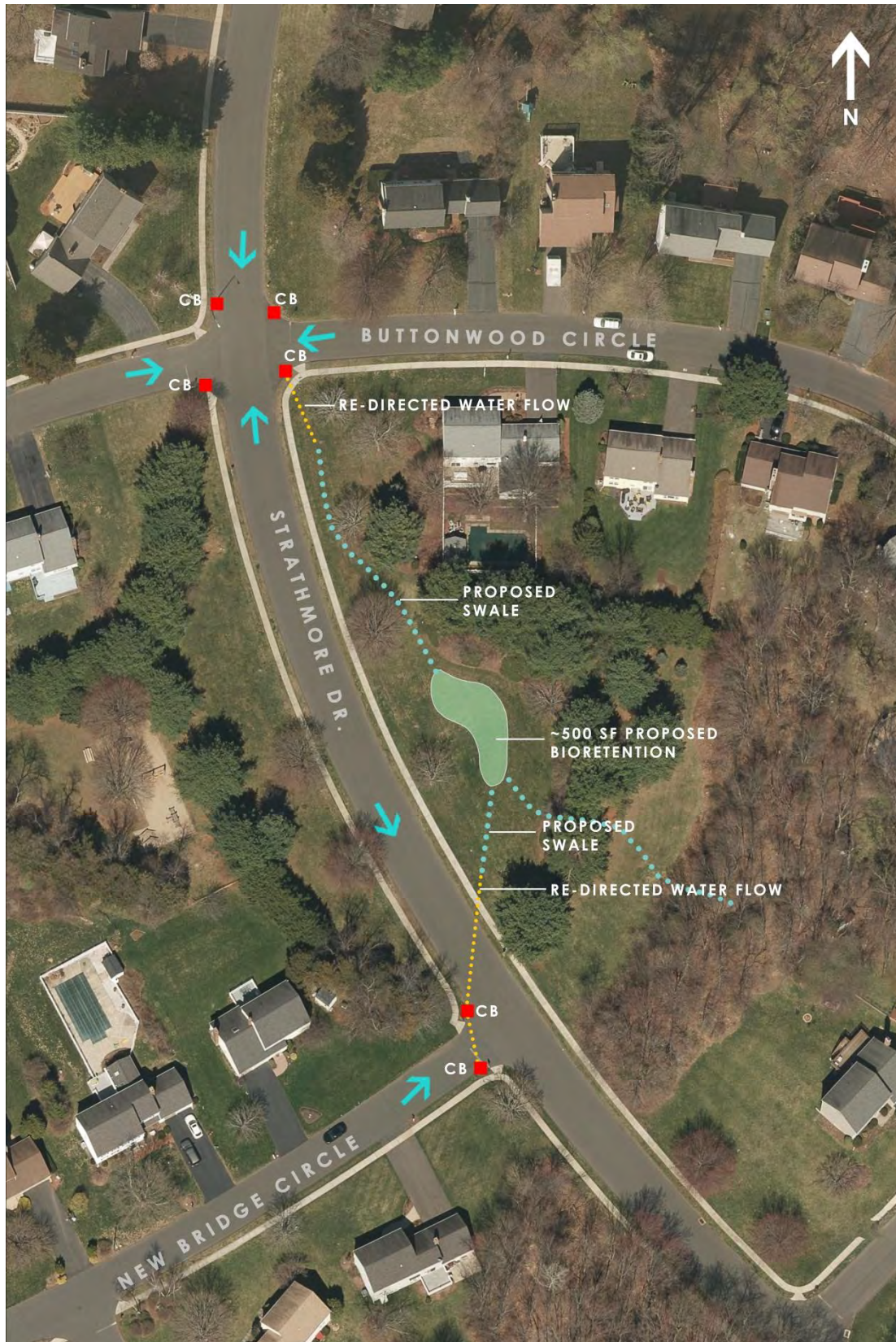
Figure 27. Proposed green infrastructure retrofits at Strathmore Drive. "CB" indicates existing catch basin. Blue arrows indicate existing surface flow patterns.
