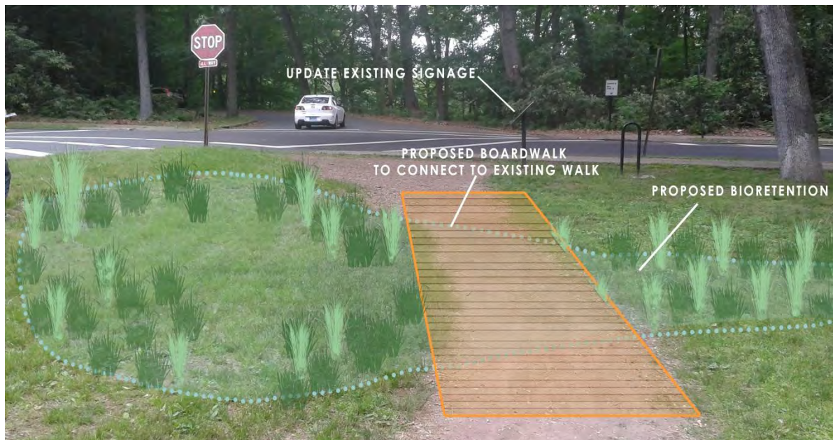
Figure 17. Proposed bioretention area and trail improvements in East Rock Park.
