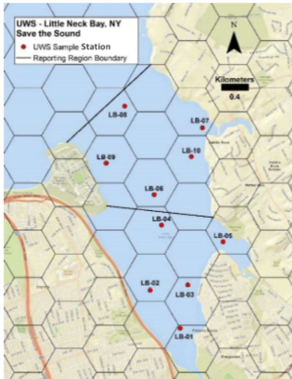
Figure 2: Hexagons overlaying Little Neck Bay, NY. Numbers indicate station locations. Eight of the hexagons overlaying embayment water do not contain stations. This is an example of how some hexagons may be eliminated from sampling for larger embayments. Criteria for eliminating hexagons include an assessment of representability of neighboring stations, hexagons which include a large proportion of land, and stations closer to Long Island Sound likely to be well-mixed and similar to neighboring stations.
