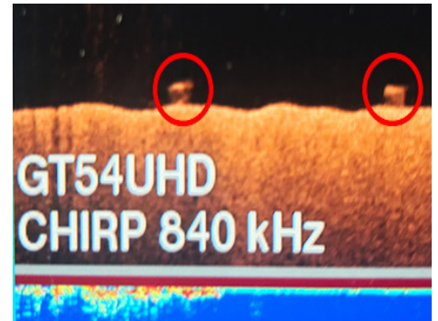
Above: The grapple system employed by Cornell Cooperative Extension (CCE) in Mount Sinai Harbor, NY. Left: CCE staff inspecting a retrieved pot on Long Island. Below: The sonar technology used to detect abandoned lobster pots on the seafloor.
