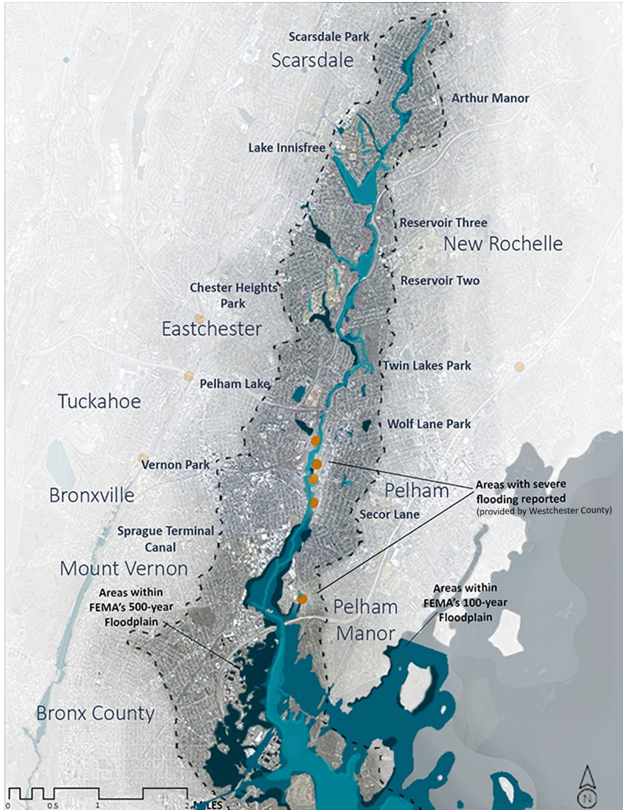
Figure 16: FEMA 100 and 500-year floodplain and reported flooding in the Hutchinson River Watershed.
